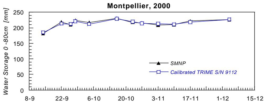
Fig. 6 : Example of water storage monitored by a calibrated TRIME compared to its equivalent estimated from SMNP data.
