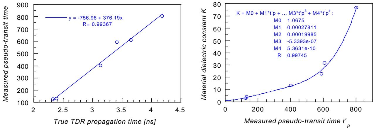
Fig. 9 : TRIME and classical TDR measurements taken in reference media of Table 2.
