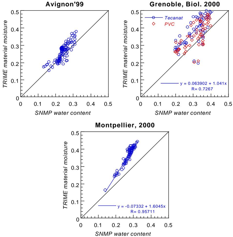
Fig. 3 : Direct comparison of measured water-contents for all dates and depths for three experimental sites.
