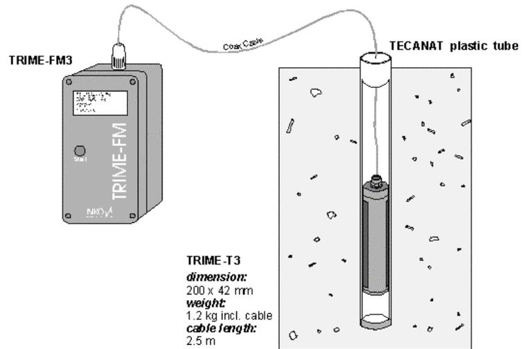
Fig. 1 : The TRIME-Tube system
