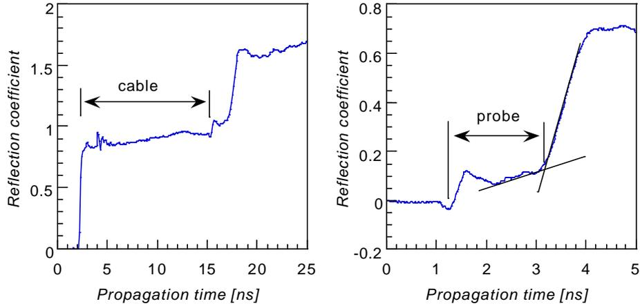
Fig. 8 : Example of TDR signals acquired with a Tektronix on a T3-Probe. Water-saturated glass beads. Left : complete signal, right : detail of the useful part corresponding to the propagation in the probe itself.
