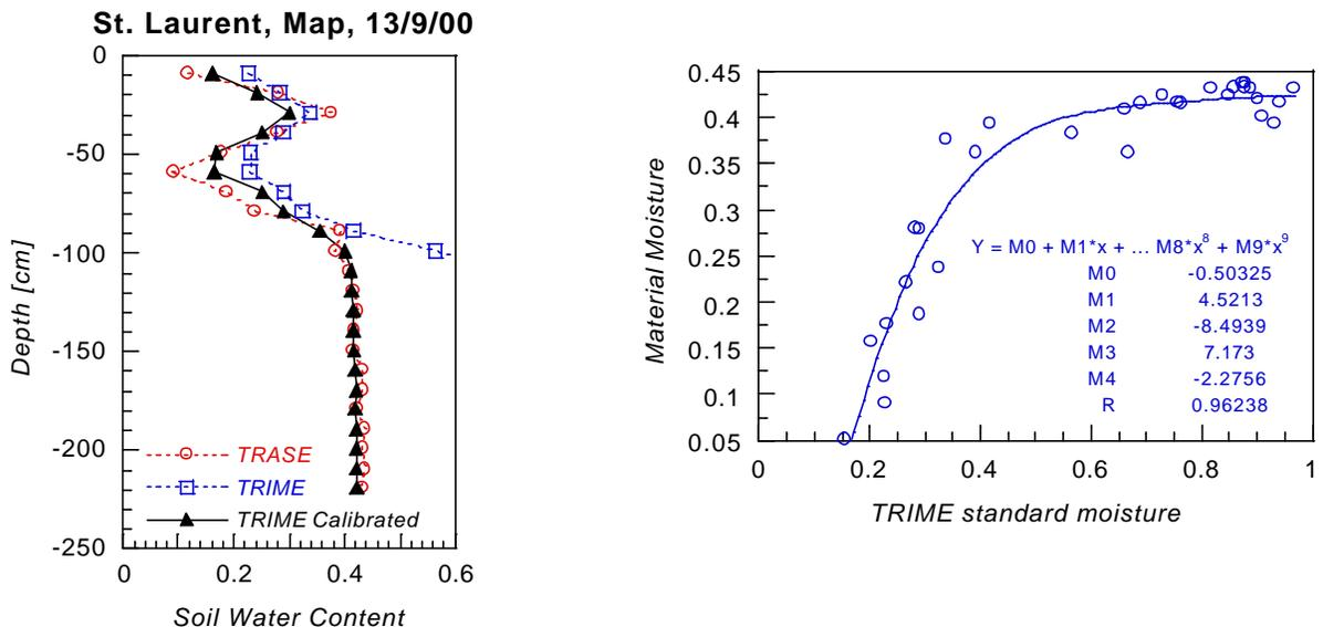
Fig.10 : Calibration of the TRIME-tube measurements at St. Laurent de la Prée (see text).
