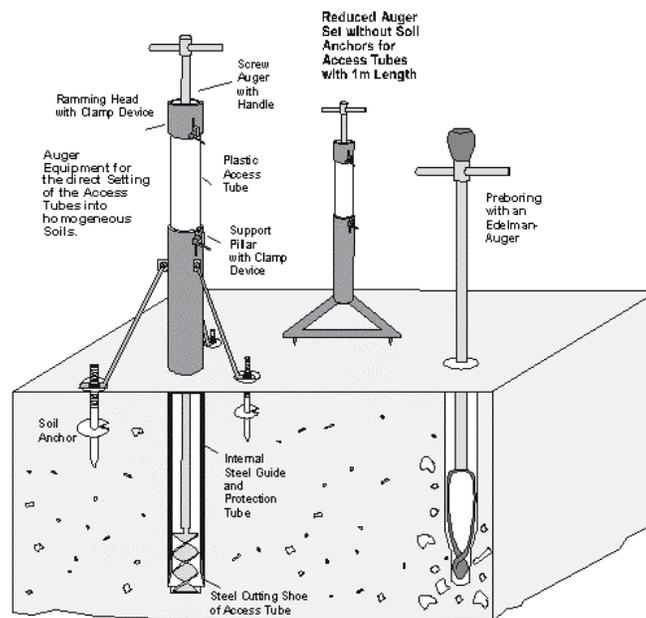
Fig. 2 : TRIME tube installation kits.
