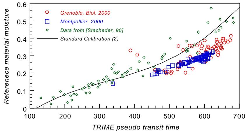
Fig. 4 : Deviation of our results on two sites from the TRIME standard calibration curve (2)
