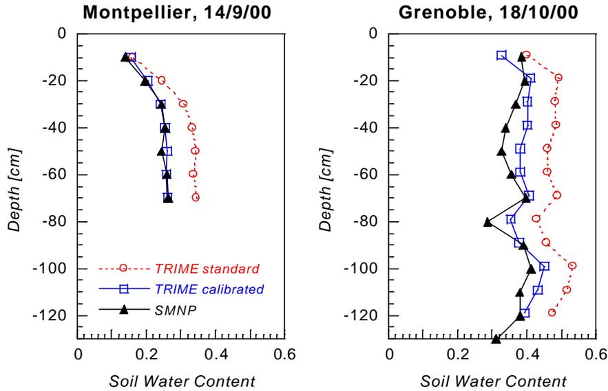
Fig. 5 : Examples of comparison of soil moisture profiles before and after TRIME calibration.
