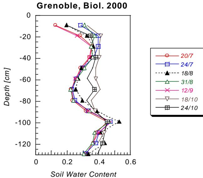
Fig. 7 : Example of water profile monitoring with a TRIME-tube system.
