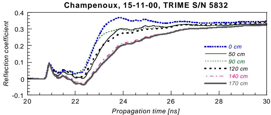
Fig. 11 : Examples of TDR-waveforms acquired on the T3-probe in a tube in the Champenoux forest.
