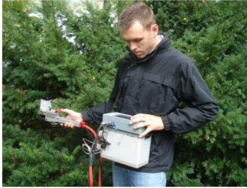
iFL - integrated fluorometer with absorbance measurement.
